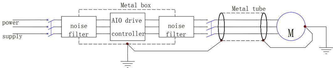
Fig 4.16 better anti-interference measure
