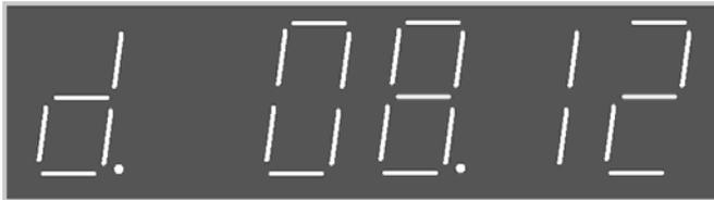
The above picture show: 8 month 12 day. “d” is the abbreviation of day. When need of modify, press the enter button. The figure in the lowest order start to flash, use the left or right button to select the figure required for modification. The selected figure starts to flash. Then use up or down button to modify the figure, press the enter button to confirm the modification.
