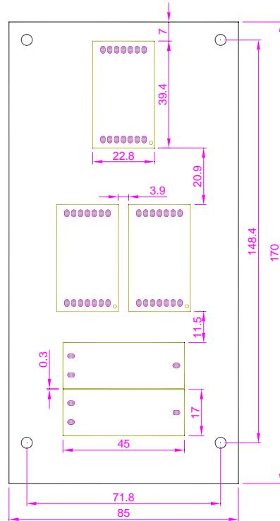
Fig 6.30 SM-04-VRJ installation dimension
