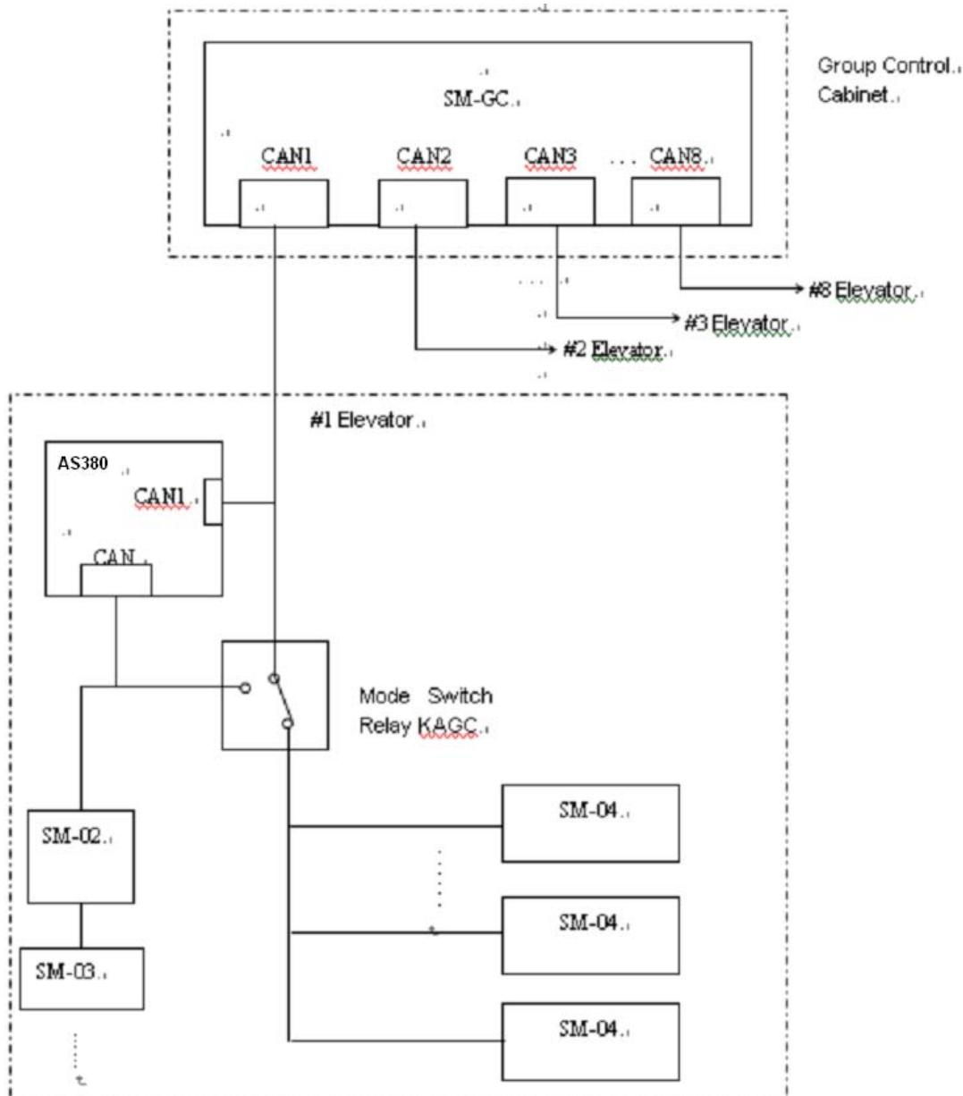
Fig 6.28 System structure.
