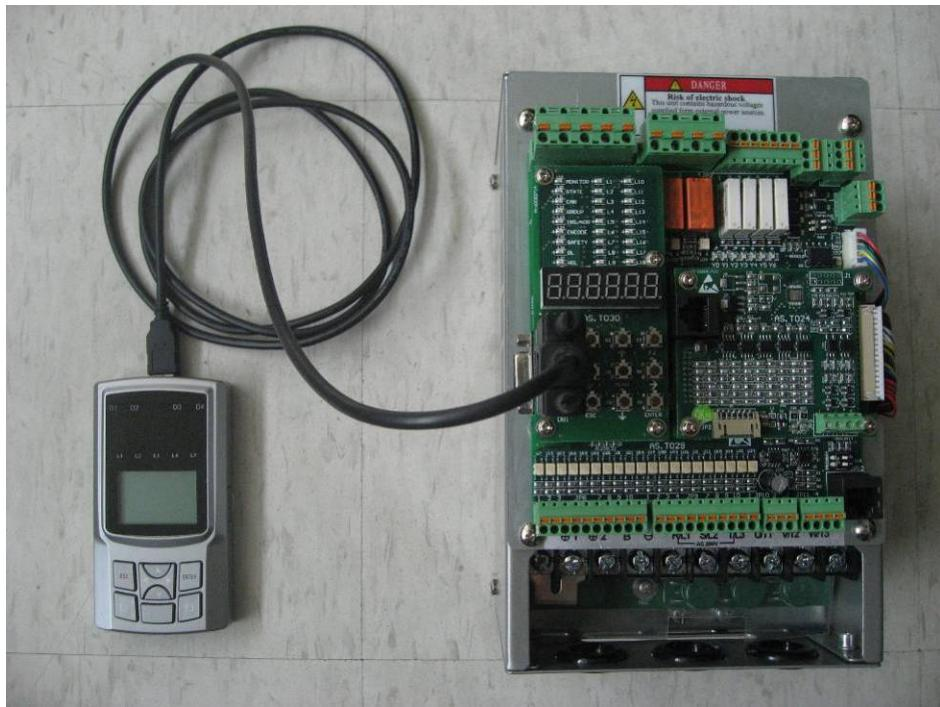
Fig. 5.3 the integrated device and handheld operator
