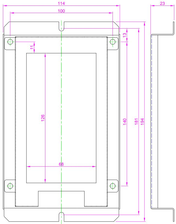
Fig 6.26 SM-04-VL/B3 installation dimension
