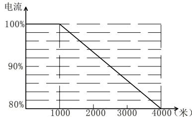
Fig 1.4 the diagram about the relation between the rated output current and altitude
