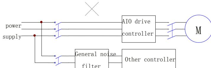
Fig 4.8 the wrong setting of noise filter at the side of power supply
