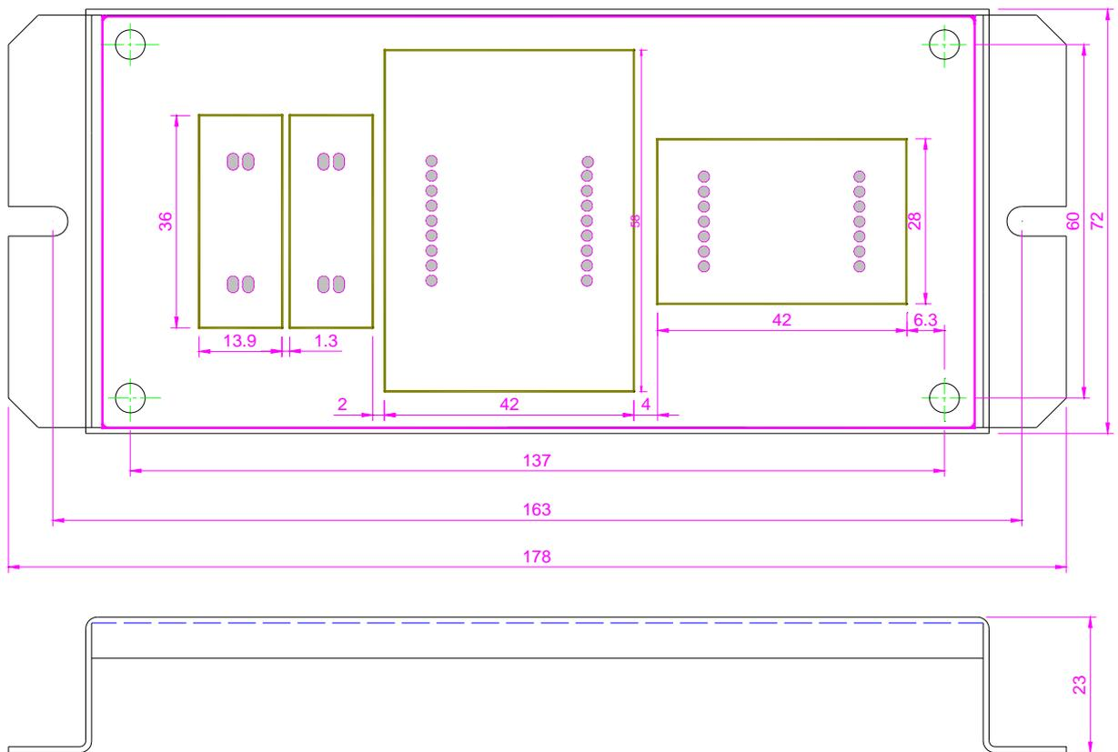
Fig 6.28 SM-04-VSD installation dimension
