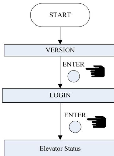
Picture 5.5 operations from power on to elevator status window
