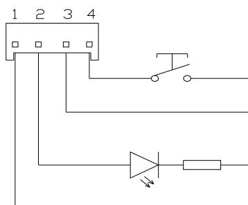
Fig 6.10 instruction button and indicator lamp wiring diagram
