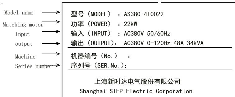
Fig 1.2 Nameplate description of elevator integrated drive controller
