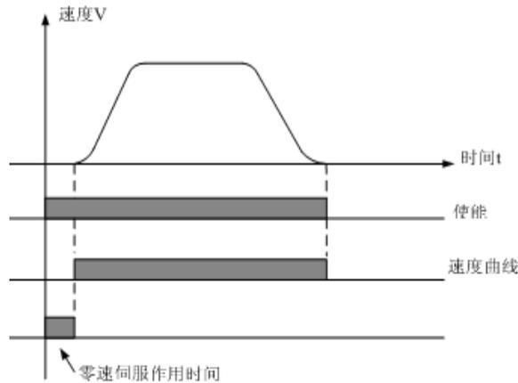
Fig 7.4 the action time of zero servos
