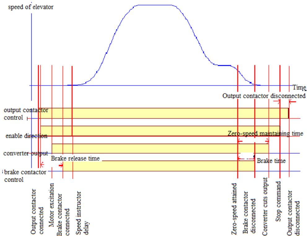
Diagram 8.2 Adjustable Timing Sequence Diagram
