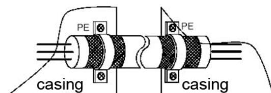
Figure A2.2 Correct Shield Grounding Method
