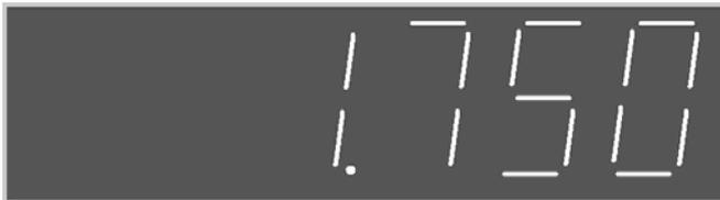
This menu display the current running speed of elevator, the unit is M/S. as above fig, the current speed displayed is 1.75m/s
