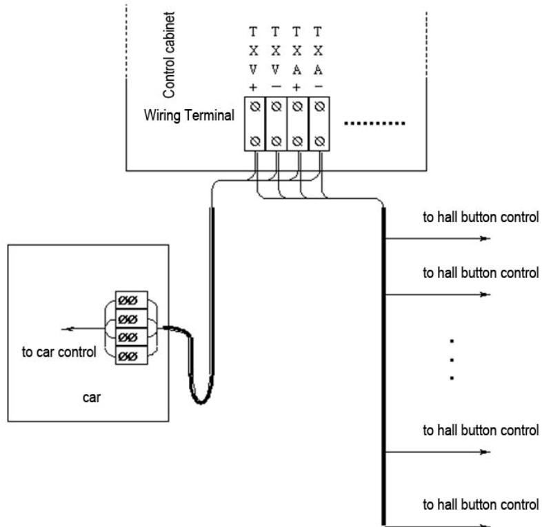
Fig 4.2 hoist way and accompanying cable arrangement
