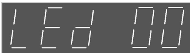
Use up and down button to select the definition code of 18 LED indicator light L1-L8. press enter button to confirm. The LED indicator light will change as per the code definition. The definition code of L1-L8 is as following table 5.5
