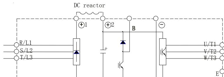
Fig 4.11 external connected DC reactor wiring
