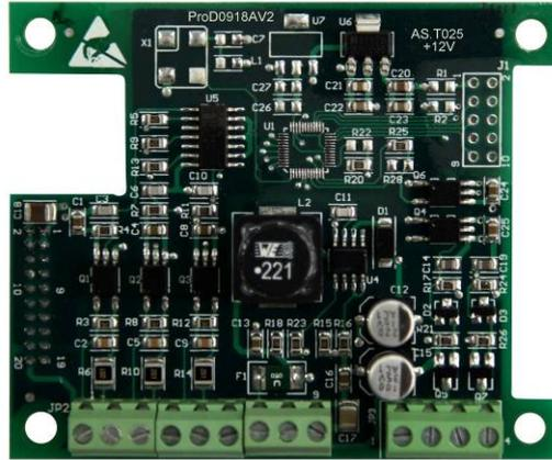
Fig 4.18 ABZ incremental 12v PG card terminal layout
