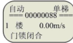
F187 set as 0: to display the running times of elevator
