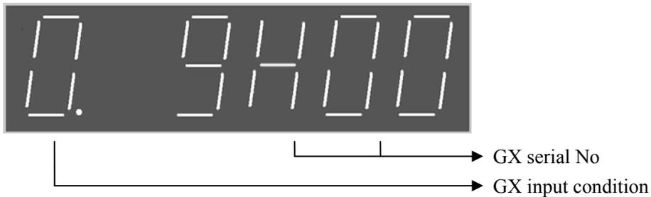
The above figure show the GX0 has no input, press up or down to select GX serial no the serial no start from 0 to 15. After finished the selection of corresponding serial no GX, the figure in the highest order show the input to this input terminal is valid or not. (0 represents no valid input. 1 represent valid input)
