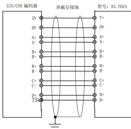
Fig 4.2.2 the wiring of sin/cos differential output signal of encoder
