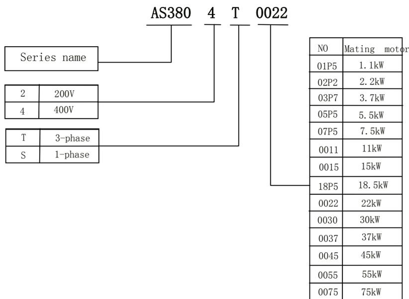
Fig 1.1 Model illustration of elevator integrated drive controller
