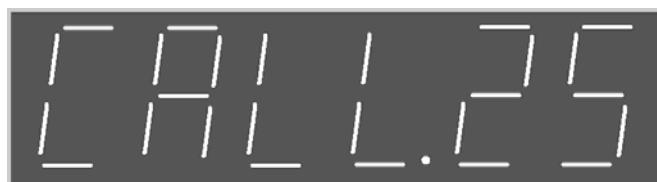
Use up and down button to select the floor needed to register the instruction, press the enter button, to register the instruction.
