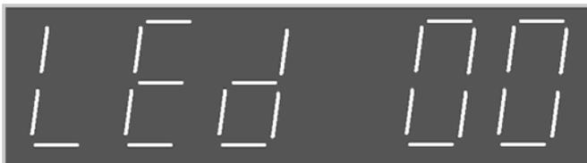
Use up and down button to select the definition code of 18 LED indicator light L1-L8. press enter button to confirm. The LED indicator light will change as per the code definition. The definition code of L1-L8 is as following table 5.5
