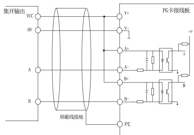
Fig 4.20 the wiring of encoder push-pull signal
