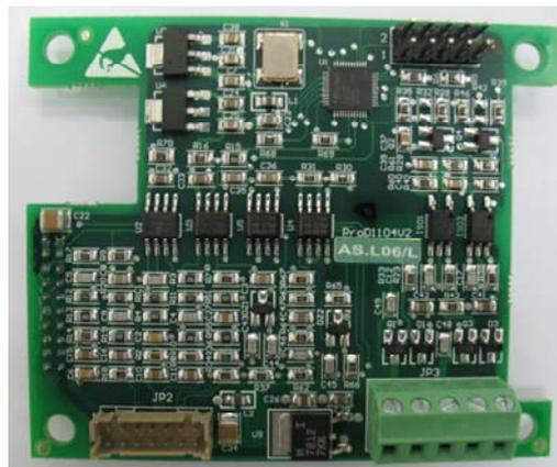
Fig .4.24 Endat absolute value PG card terminal layout
