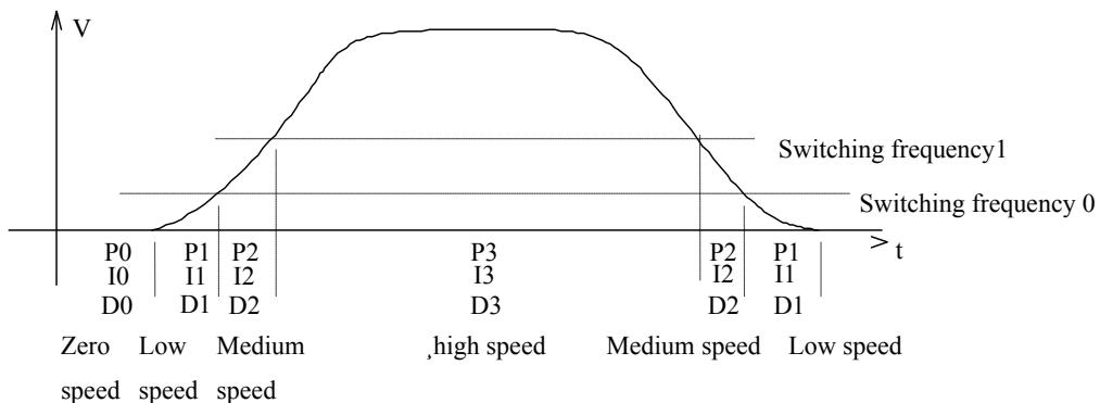
Diagram 8.3 Elevator operation curve segment PI control chart
