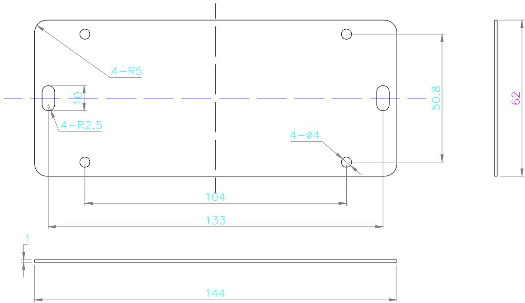
Fig 6.4 car top extension board installation dimension
