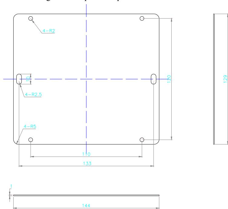
Fig 6.2 car top control baseboard installation dimension
