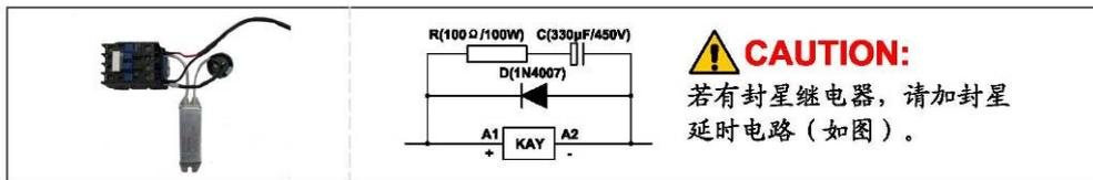
Fig 1.5 sealing star delay circuit tag
