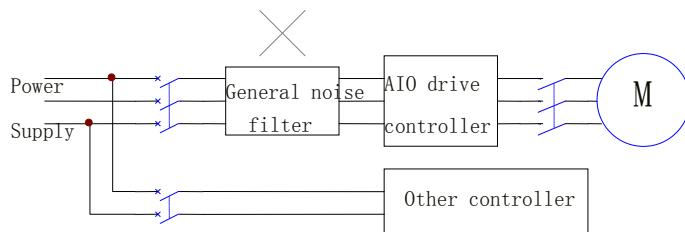
Fig 4.9 the wrong setting of noise filter at the side of power supply
