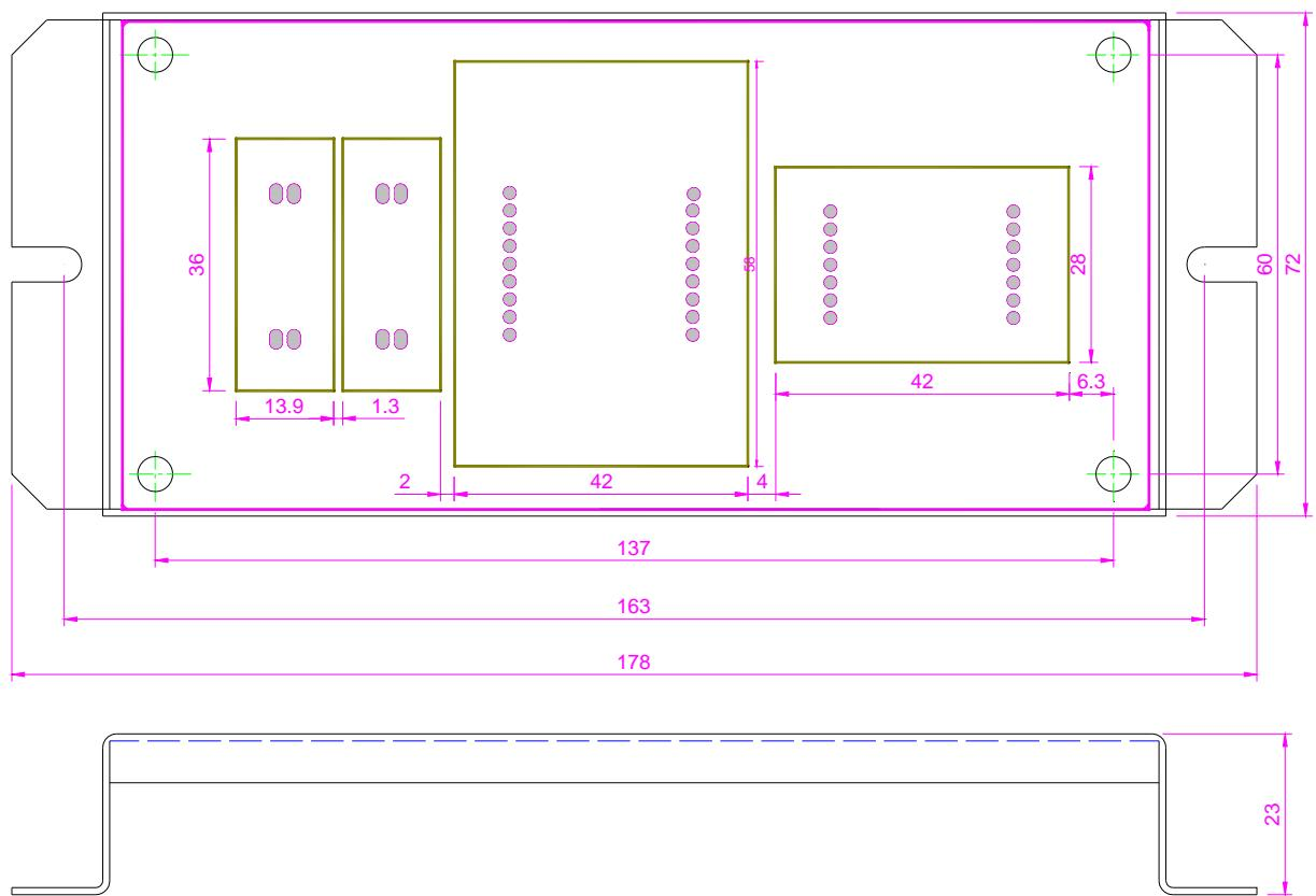
Fig 6.28 SM-04-VSD installation dimension
