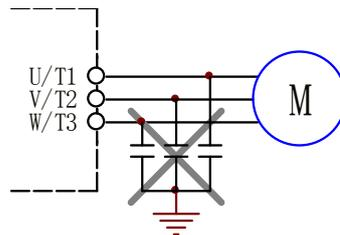
The schematic diagram of no connection of capacitor at the output side of integrated drive controller
