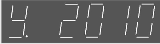
The above picture show: the year 2010, “Y” is the abbreviation of year, when need to modify, press enter button, the figure in the lowest order start to flash, use left or right button to select the figure required for modification. The selected figure start to flash. Then use up or down button to modify the figure ,press the enter button to confirm the modification.
