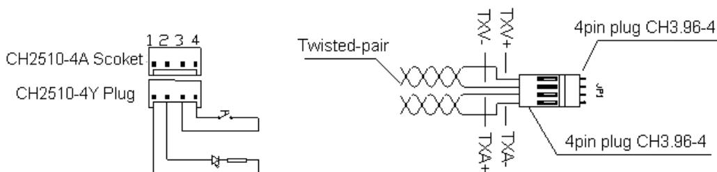
Fig. 6.31 Connection of the Push Button Lines
