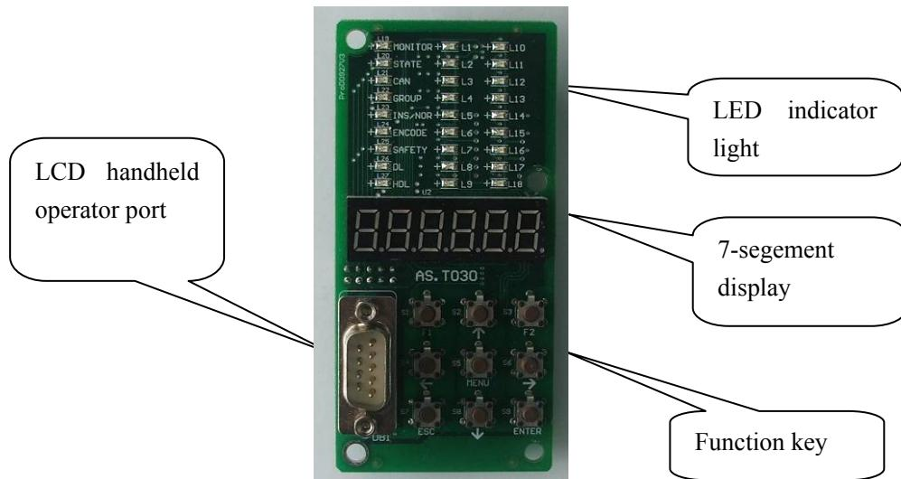
**Fig 5.1 7-segment operator**
