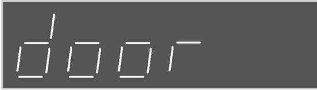
When Bit 3 of parameter F165 (door open./close control ) is set to 1, the door open/close function of LED operator is activated. Press the F1 at this interface to make system output the door open signal. Press F2 to make the system output door close signal.
