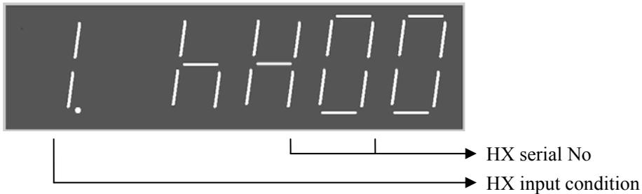
The above figure show: HX0 has no input. Press up or down to select HX serial No. serial no start from 0-15. after finishing the selection of corresponding serial no HX, the figure in the highest order show the input to this input terminal is valid or not ( 0 represent no valid input , 1 represent
