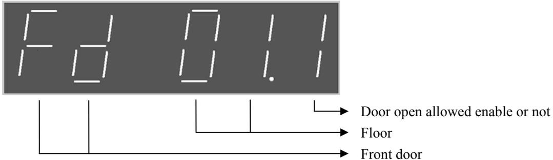
The above picture mean: shield 1 floor front door open allowed. Fd is the abbreviation of Front door. Press the up and down button to browse the front door open allowed parameter of corresponding floor. Press the enter button to make modification. The figure in the lowest order starts to flash, use up or down button to modify the figure into 0 or 1. Press the enter button to confirm the modification (0 is to shield front door open allowed function, 1 is to allow front door open function)
