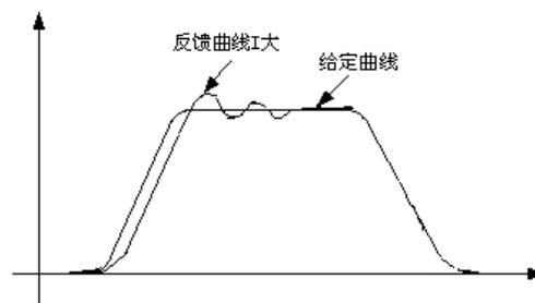
Fig 7.2 effect of integral constant I upon feedback
