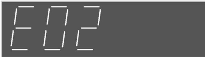
The menu shows the program version of control part of integrated unit. The screen will display the program version E02 of the control part one second later, as per the above picture. Then the words VER 2 and E02 will alternatively display, each of which will last for 1 second.
