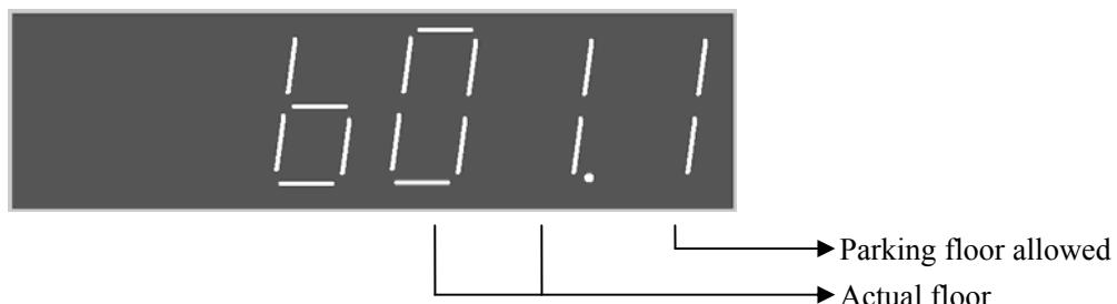
Use up and down button to select the floor need to modify. Please note, the floor mentioned here is the actual floor ( or the control floor) press the enter button. The selected value start to flash, press the up and down button to set the value. press the enter button to confirm, in which 1 mean parking allowed, 0 mean parking prohibited.
