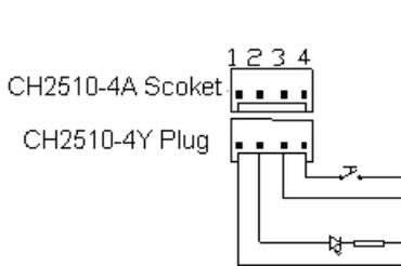
Fig. 6.31 Connection of the Push Button Lines
