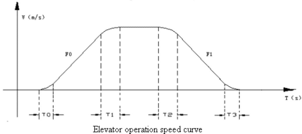
Figure 8.4 Elevator Operation Curve
