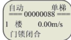
F187 set as 0: to display the running times of elevator
