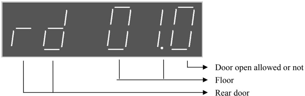
The above picture mean: shield 1 floor rear door open allowed. Rd is the abbreviation of rear door. Press the up and down button to browse the rear door open allowed parameter of corresponding floor. Press the enter button to make modification. The figure in the lowest order starts to flash, use up or down button to modify the figure into 0 or 1. Press the enter button to confirm the modification (0 is to shield rear door open allowed function, 1 is to allow rear door open function)
