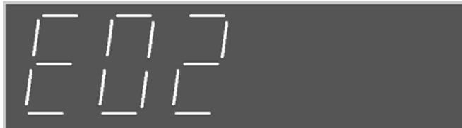
The menu shows the program version of control part of integrated unit. The screen will display the program version E02 of the control part one second later, as per the above picture. Then the words VER 2 and E02 will alternatively display, each of which will last for 1 second.
