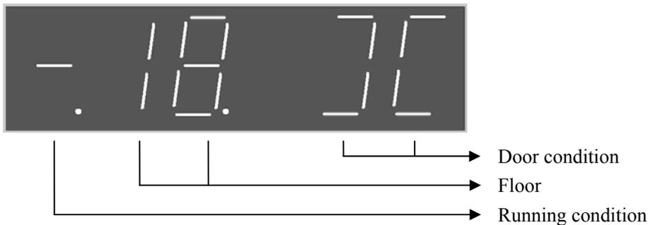
This menu will display the basic condition of elevator, including running condition, floor located, and door condition.
