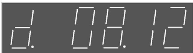
The above picture show: 8 month 12 day. “d” is the abbreviation of day. When need ot modify, press the enter button. The figure in the lowest order start to flash, use the left or right button to select the figure required for modification. The selected figure starts to flash. Then use up or down button to modify the figure, press the enter button to confirm the modification.
