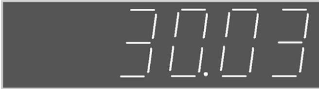
The menu shows the program version of drive part of integrated unit. The screen will display the program version 30.03 after 1 second waiting. Then the word ver1 and 30.03 will alternatively display, each of which will last for 1 second
