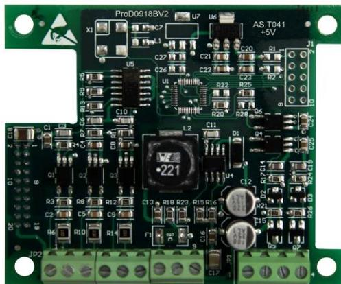
Fig 4.23 ABZ incremental 5V PG card terminal layout
