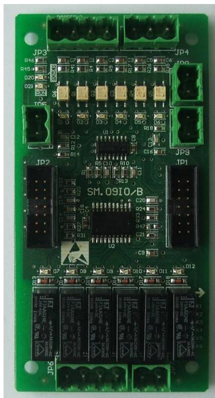
Fig 6.3 car top extension board outside view
