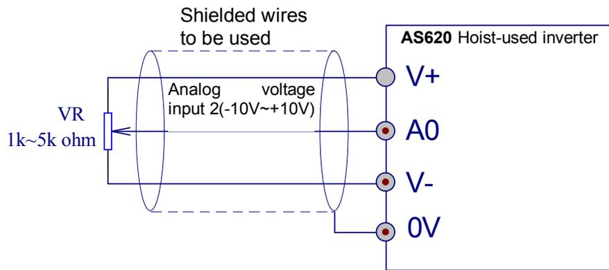
Fig- 4.18 Analog input signal shielded wire wiring
