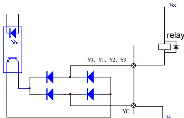
Fig- 4.20 Circuit of open collector outputs
