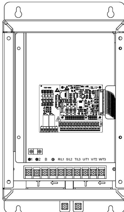
Fig-. 4.2 Internal view of inverter
