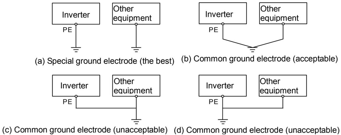
Fig- A.6 Schematic for special ground electrode
