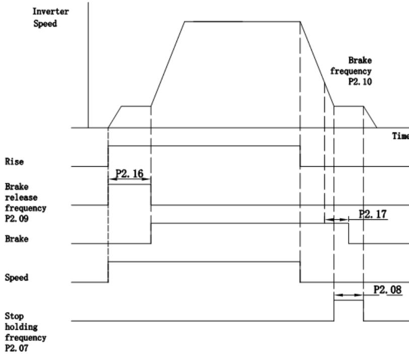
Fig- 6.3 fixed torque start rise
