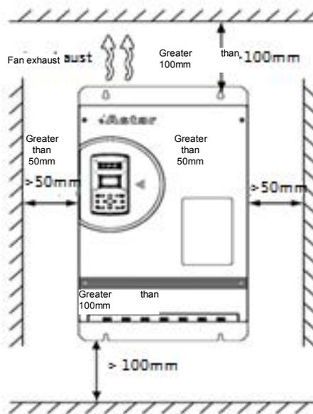
Fig-. 3.1 Schematic of spacing of inverter installation
