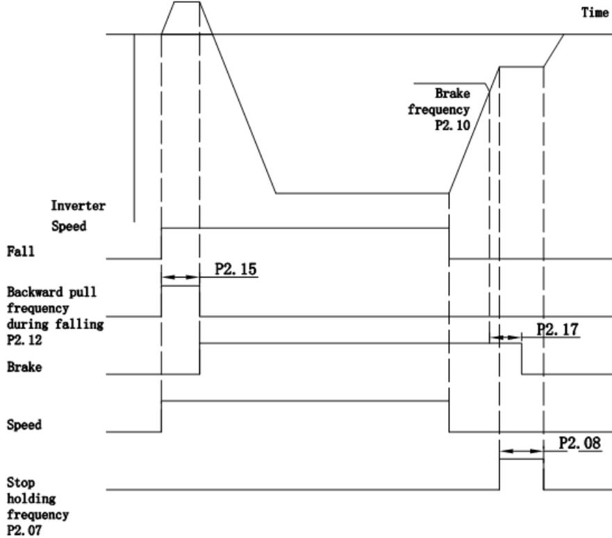
Fig- 6.4 fixed torque start fall
