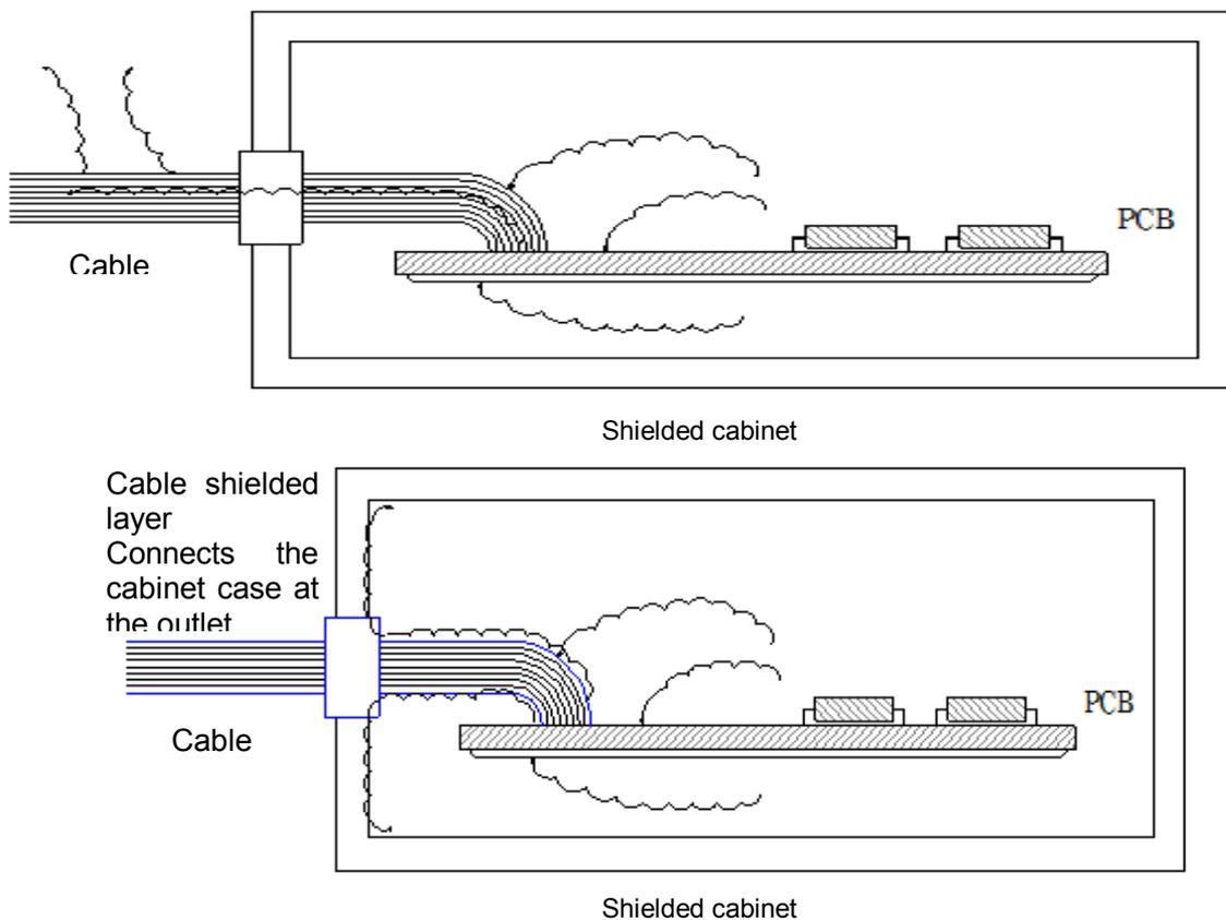
Fig- A.10 Suppression of radiation by connecting the cable shielded layer to the ground of the case
