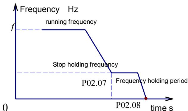
Fig- 7-5 stop holding frequency diagram
