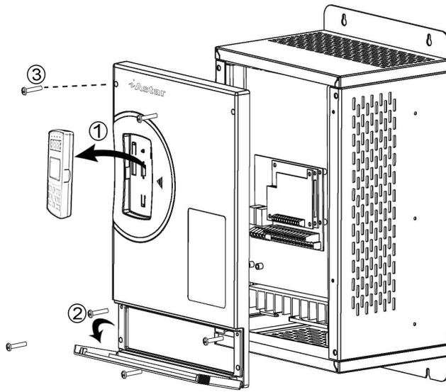
Fig-. 3.6 Removal of front panel
