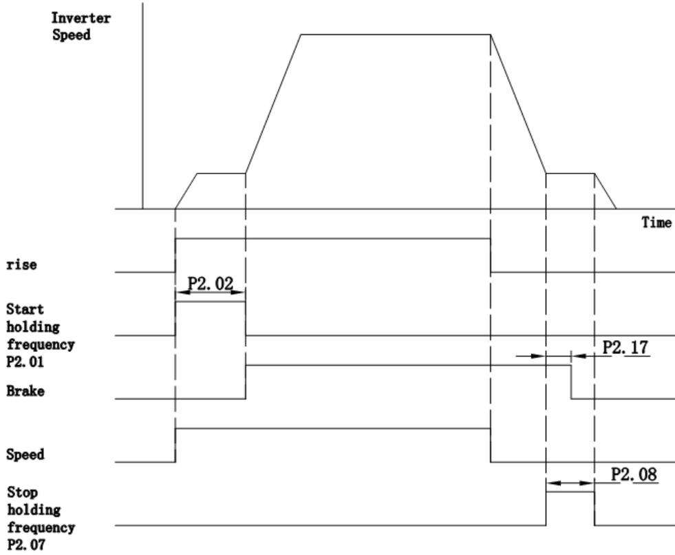
Fig--6.1 positive/nergative torque start rising
