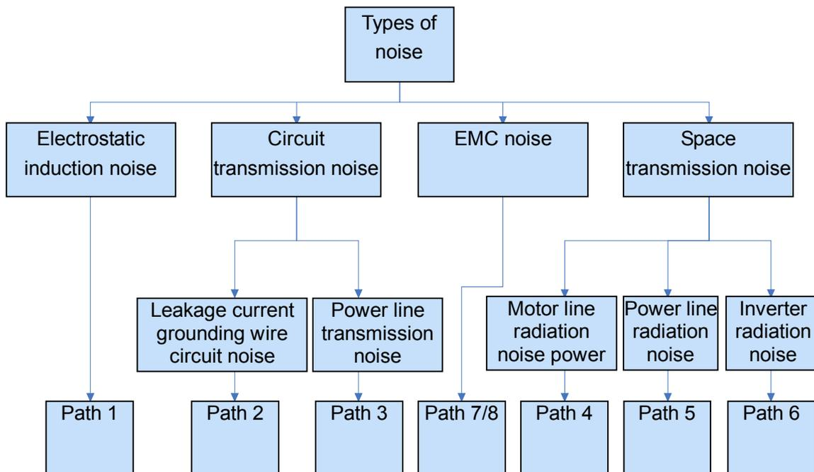
Fig- A.1 Schematic of the types of noise
