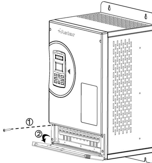
Fig-. 3.5 Opening wiring cap
