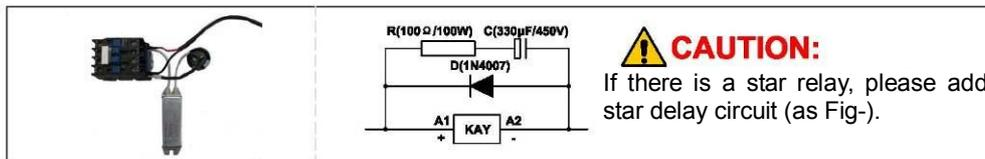
Fig- 1.5 Hint sign of star delay circuit
