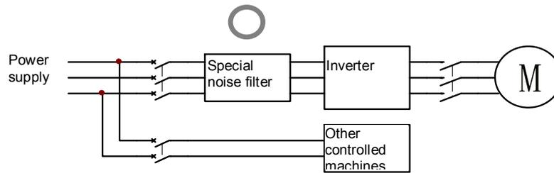
Fig- 4.7 Noise filter on the power supply side
