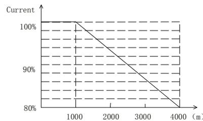
Fig-1.4 Relation diagram between rated output current and altitude of inverter
