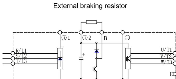
Fig- 4.12 External braking resistor wiring
