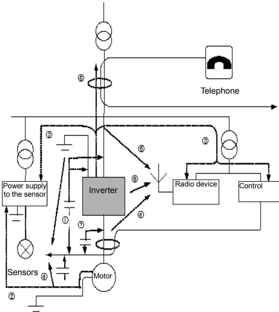
Fig- A.2 Noise transmission schematic
