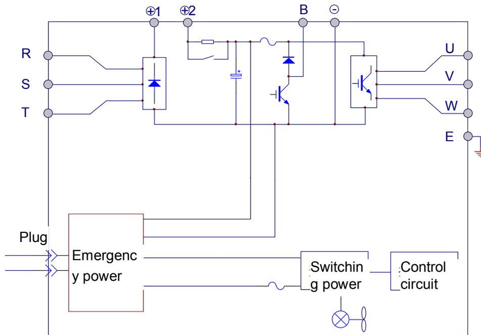
Fig- 4.4 Main circuit conFig-urations
