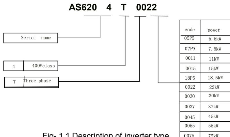
Fig- 1.1 Description of inverter type
