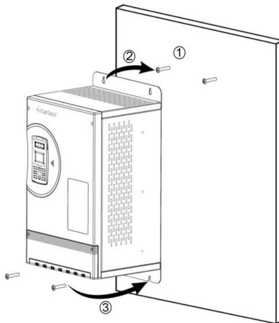
Fig-. 3.2 Diagram of inverter installation order
