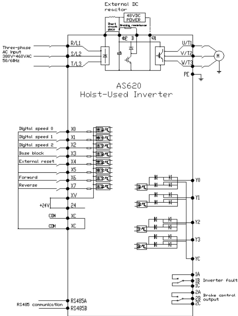
Fig- 4.3 Wiring diagram of inverter terminals
