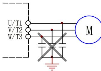
Fig- 4.13 Never connect capacitor on the output side of the Inverter
