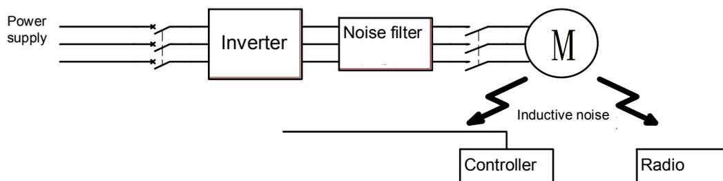
Fig- 4.14 Connection of noise filter on the output side of the Inverter
