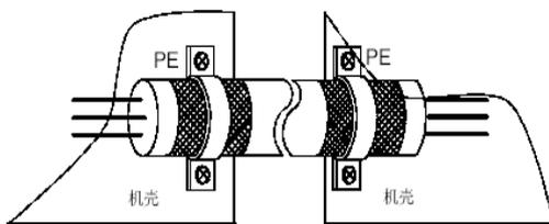
Fig- A.4 Correct shielded grounding method
