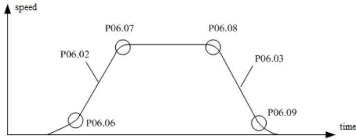
Fig-7-7 S curve bv's position during motor running
