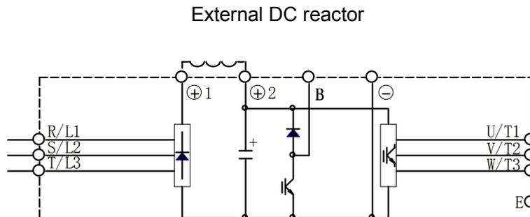
Fig- 4.11 Wiring of the external DC reactor
