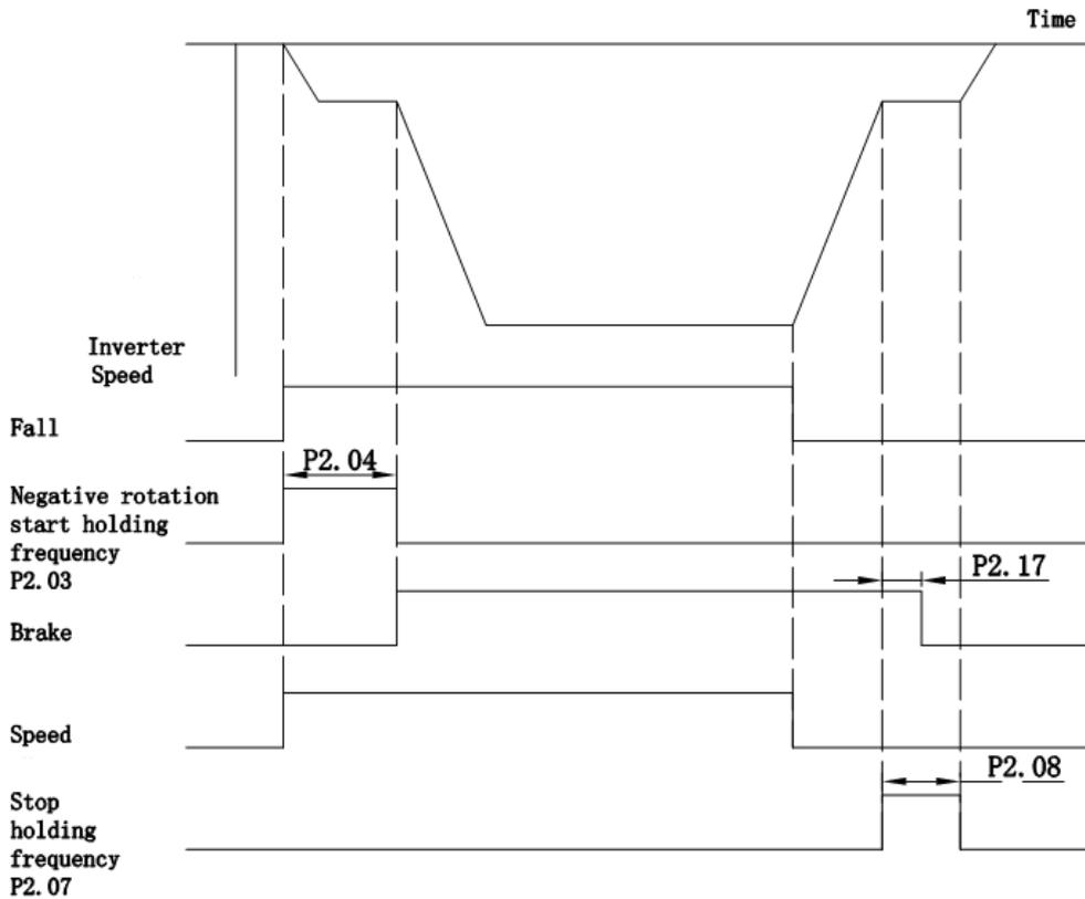
Fig- 6.2 positive/nergative torque start falling
