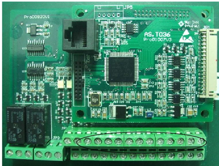
Fig- 4.17 Control circuit terminals
