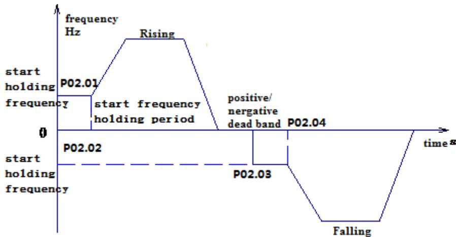
Fig- 7-1 start frequency start mode diagram
