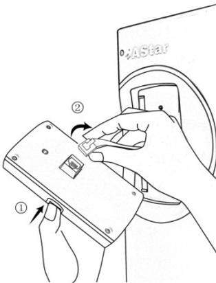
Fig-.3.4 Assembly and disassembly of operating device
