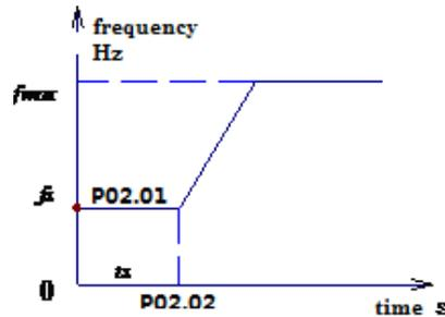
Fig- 7-3 start frequency and start time diagram
