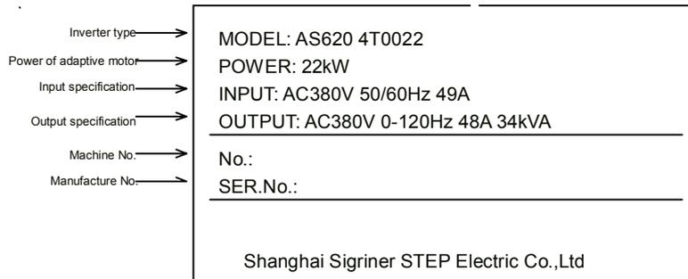
Fig-.1.2 Description of inverter name plate
