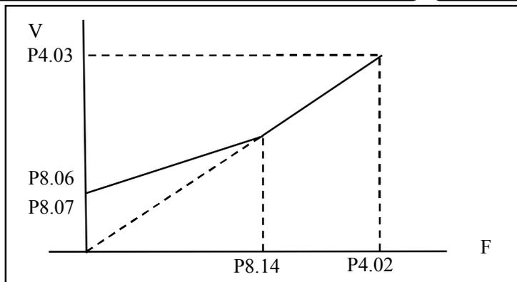
Fig- 7-9 falling start compensation frequency diagram
