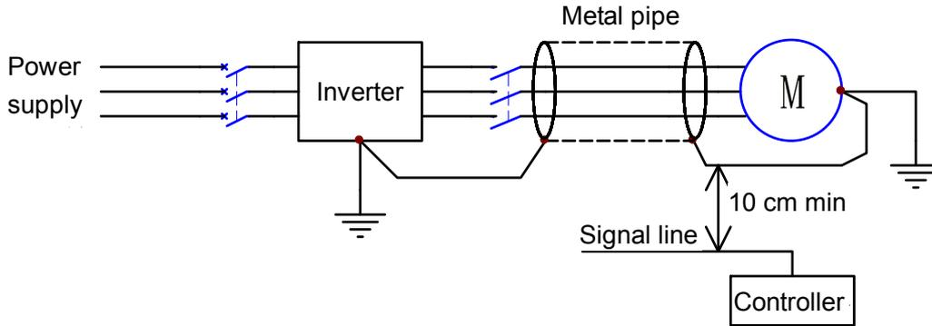
Fig- 4.15 Main circuit wiring
