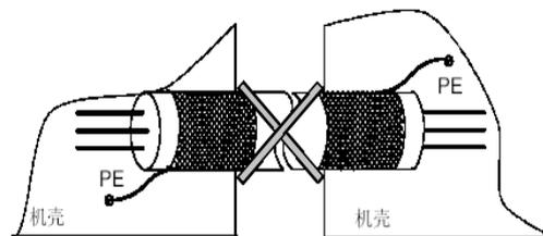
Fig- A.5 Incorrect shielded grounding method
