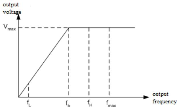
Fig- 7-8 frequency upper/lower limit diagram
