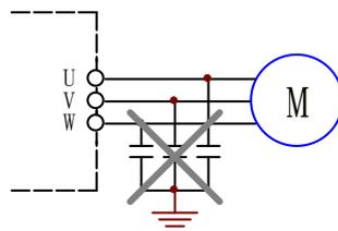
Fig-.1.3 Schematic of not connect capacitor to output side of inverter
