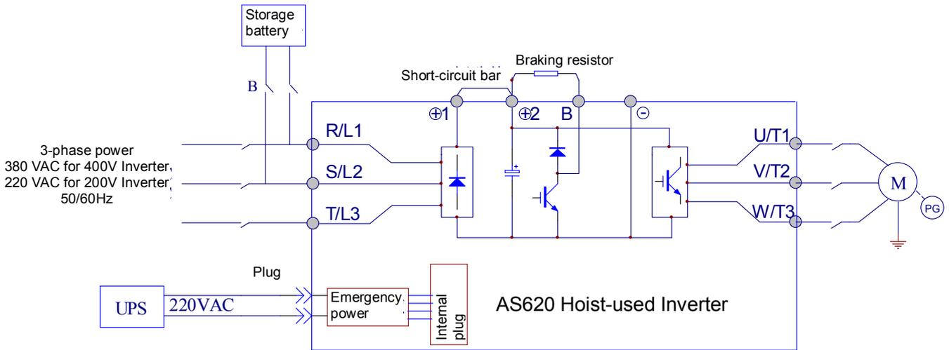
Fig- 4.6 Emergency power and storage battery connection
