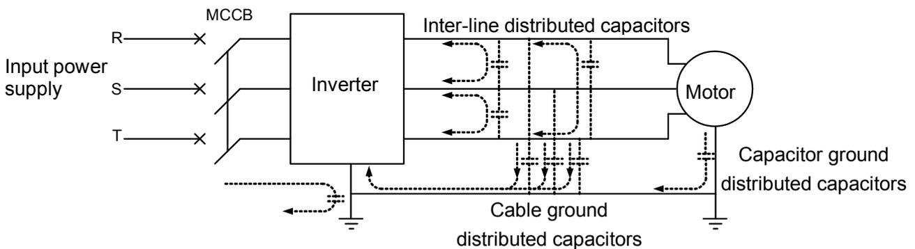
Fig- A.8 Leakage current path
