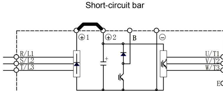
Fig- 4.10 Wiring diagram of short-circuit bar
