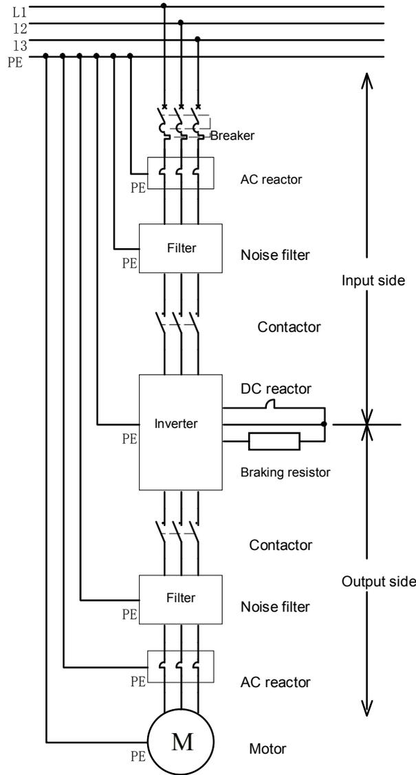
Fig-. 4.1 Connection diagram of inverter to peripheral equipments
